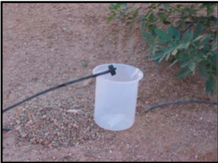
Drip irrigation spaghetti tubing and emitter. Auditing drip irrigation by measuring drip rate.
